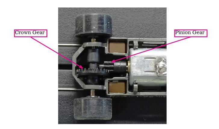
Here's an example of how to determine what your car's gear ratio would be. If your crown gear on the rear axle has 24 teeth and your pinion gear on the motor has 8 teeth, your gear ratio would be 3:1. Here's the equation and how to do math,
